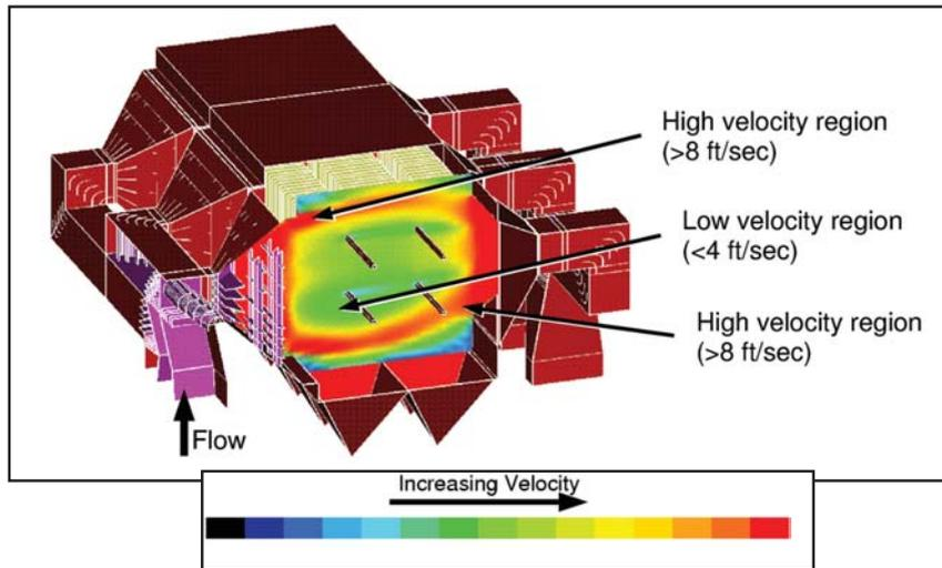
Figure 5 - Baseline flow patterns through ESP
