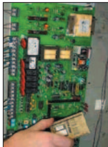
Figure 6 - Redkoh's AVC with microprocessor module removed
