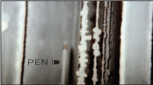
Figure 9: Donut type deposits on discharge electrodes
