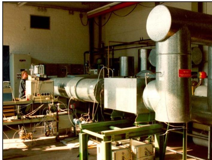
Figure 2: Steag's VGB-R302He Round-Robin certified SCR catalyst bench scale test reactor
